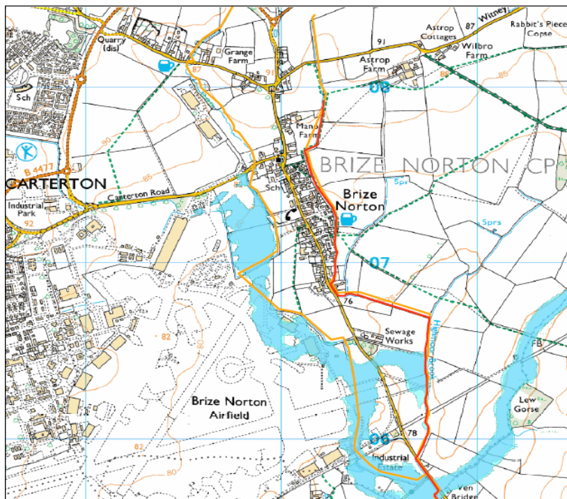
Figure 4 – Brize Norton – Flood Zone 3 (1% annual probability of occurrence) and FZ2 (0.1% annual probability of occurrence)
