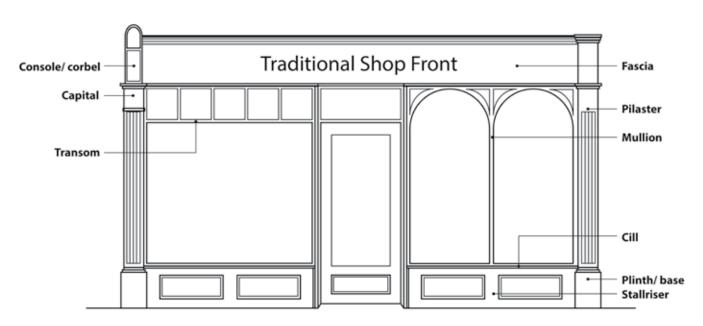
Fig. 5 The components of a traditional shop front
