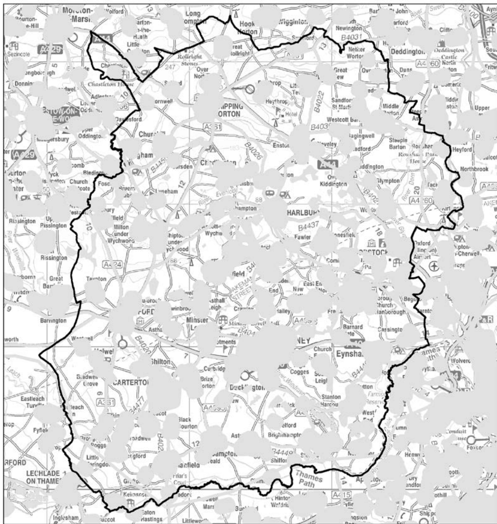
Figure 6 Small Scale Wind – Constrained areas (in grey) comprise areas within 400m of residential buildings, minimum safe distances to motorways, A and B roads and railways, minimum safe distances to major overhead transmission lines and areas of woodland and inland waters
